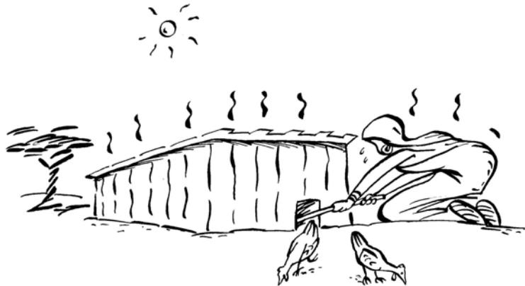
*Fig. 2.3a A badly constructed chicken house is placed in the sun with a low flat roof and no windows making it very hot and badly ventilated. It has a small door, which makes it difficult to access and clean.*
